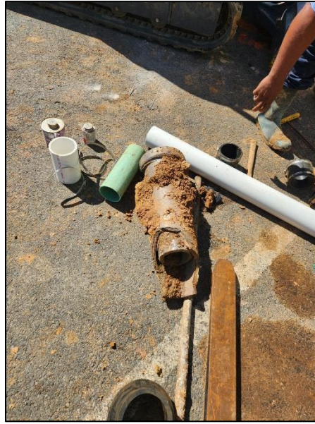
Figure 1 – Smaller diameter pipe shoved into a larger diameter pipe at the break, as described in Mr. Slone's and Mr. Powell's emails.
